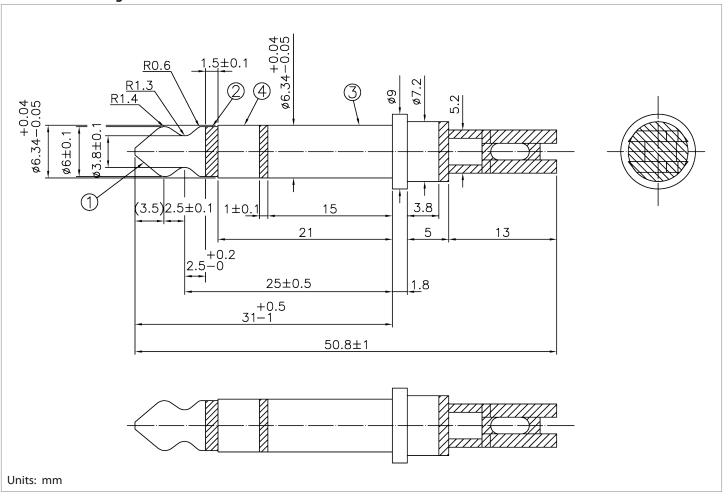
**tolerance** X: ±0.5 mm .X: ±0.3 mm .XX: ±0.05 mm applicable unless otherwise indicated in specification or on drawings
